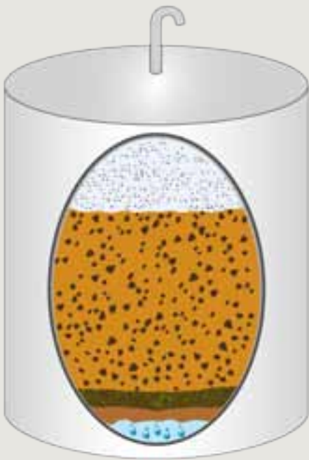
Typical storage tank contaminated with dirt, water, and microbial growth.
